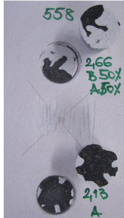
Figure 2. Cross cut test and pull off test of heat resistant coating on carbon steel (S355)
